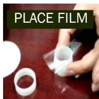
Place a circle of Mylar film on top of an XRF sample cup. This film goes on the end of the cup with the indented ring. Thermo recommends preparing the cup ahead of time, if possible.
