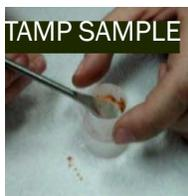
Lightly tamp the sample into the cup. The end of the pestle makes a convenient tamper.
