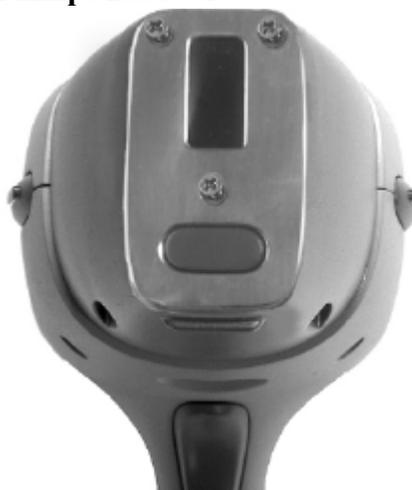
Figure 9-3. View of Face Plate and Kapton Window
