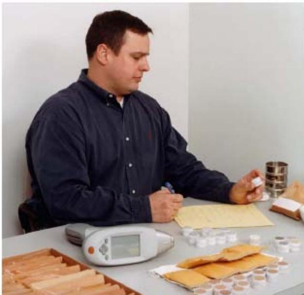
**Figure 6-13. Ex-Situ Analysis of Prepared Samples**
