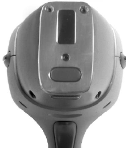
Figure 9-5. Fitting Face Plate over Proximity Button
